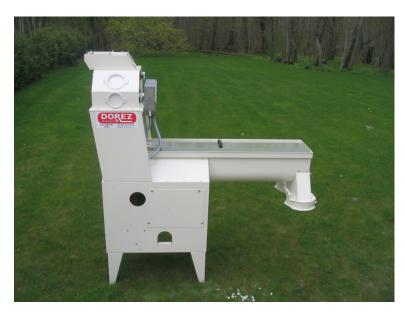
A falling box up to the weighing scale slow down the seed flow for a proper work of the scale without seed flow interaction. In **OPTION**, a by-pass up to the seed treater, allow to clean the circuit and to stop seed treatment when the quantity of treated seeds is obtained. The by-pass is activated either manually or electrically with a jack.
